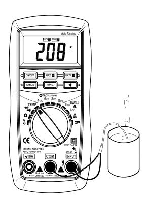
this meter can be used. Insert the black plug to the **COM** jack and the red one to the **INPUT** jack, touch the end of the temperature sensor to the area or surface of the object for measurement.
