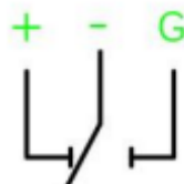
Figure 6-2 Schematic Diagram of the Relay Alarm Output Module
