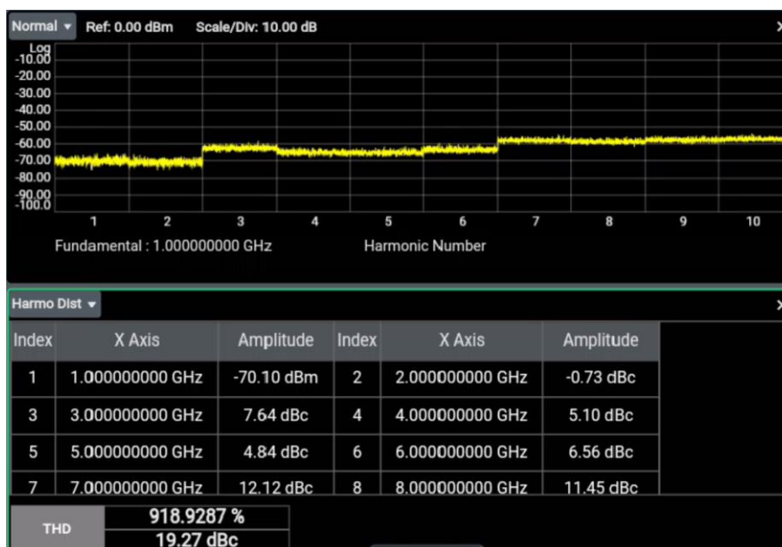
Figure 5.7 Harmonic Distortion Measurement Interface
