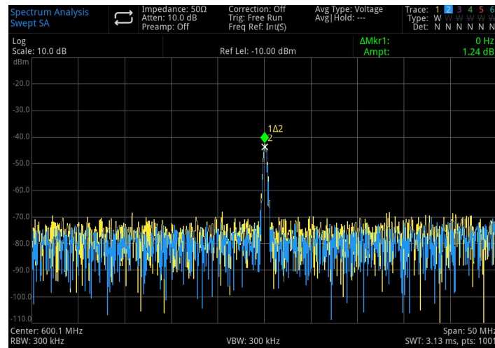
Figure 3-17 Component of Harmonic Distortion
