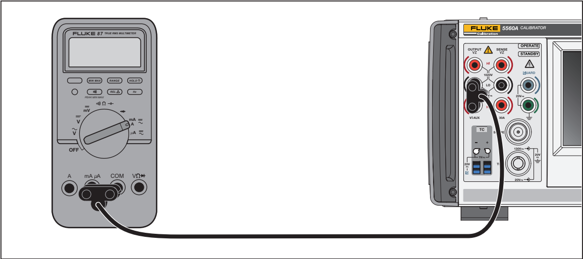
Figure 7. DUT Connection: DC Current/AC Current <3.1 A
