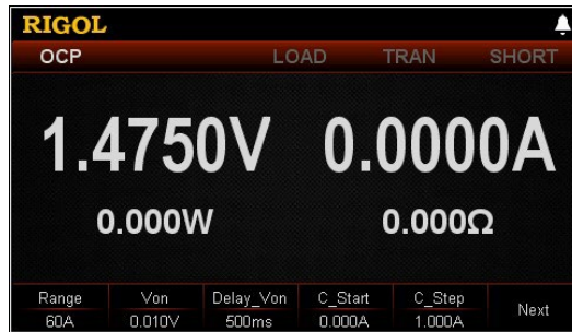
Figure 2-30 Main Interface of OCP Test Function
