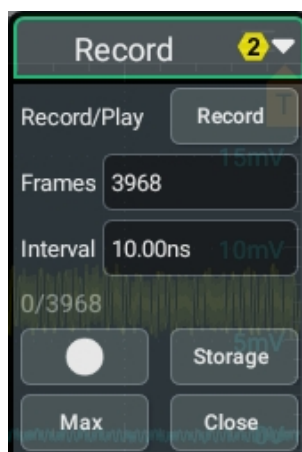
Figure 20.2 Minimized Window of the Record Operation Interface
