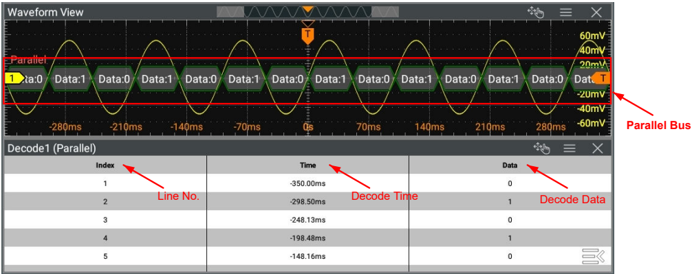
Figure 18.3 Parallel Decoding Event Table
