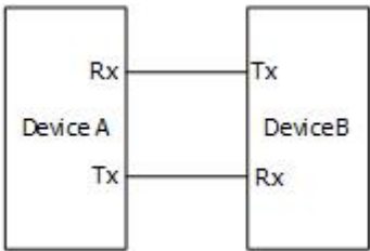
Figure 18.4 Schematic Diagram of RS232 Serial Bus
