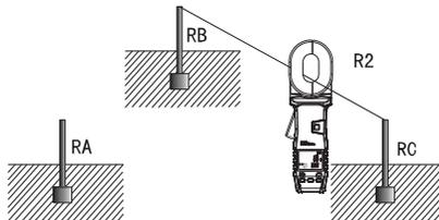
Step 3: Connect RC and RA through a test lead, then read the third data R3 from the clamp meter, see the figure below:
