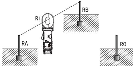
Step 2: Connect RB with RC through a test lead, then read the second data R2 from the clamp meter, see the figure below:
