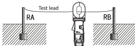
The resistance measured by the clamp meter = Resistance of RA + Resistance of RB + Resistance of test lead, that is,  $R_T = R_A + R_B + R_L$
