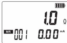
In data viewing mode, long press “**MEM**” to enter data deletion mode, short press “**AL**” to delete the data stored, and then short press “**SET**” to undelete the data.
