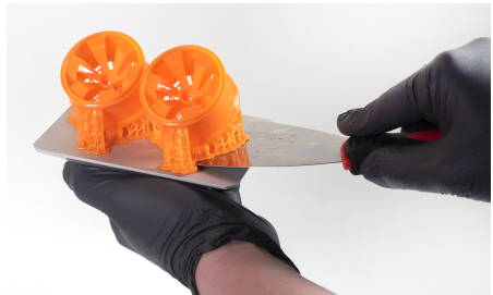
Removing a printed object with a metal spatula
