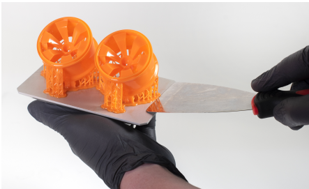
Removing a printed object with a metal spatula
