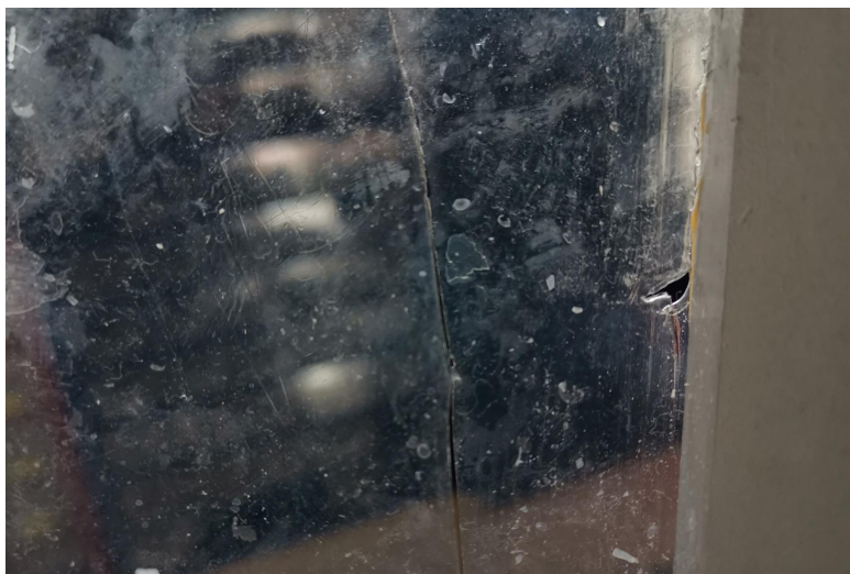
An extreme case of FEP film damage
