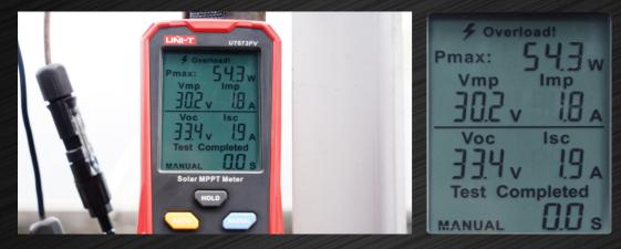
A single measurement that displays all essential test values can significantly enhance work efficiency.
