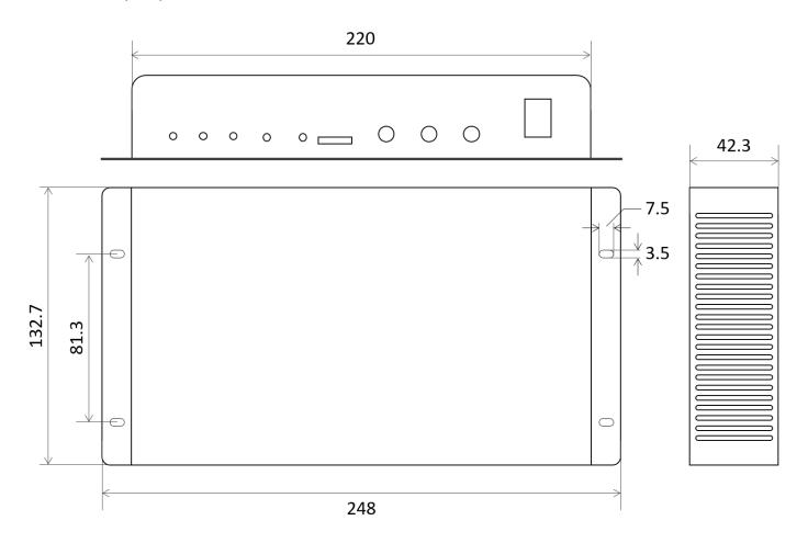
Tolerance: ±0.3 Unit: mm
