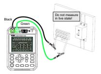
Figure 9.3.4.3 Wire connection of low resistance measurement
