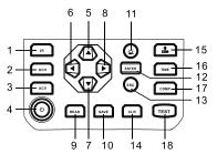
Fig. 6.1 UT512D Functional buttons
