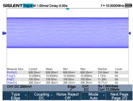
SHS800X/SHS1000X series can measure all sampled data points up to 12 Mpts. This ensures the accuracy of measurements while the math co-processor decreases measurement time and increases ease-of-use.
