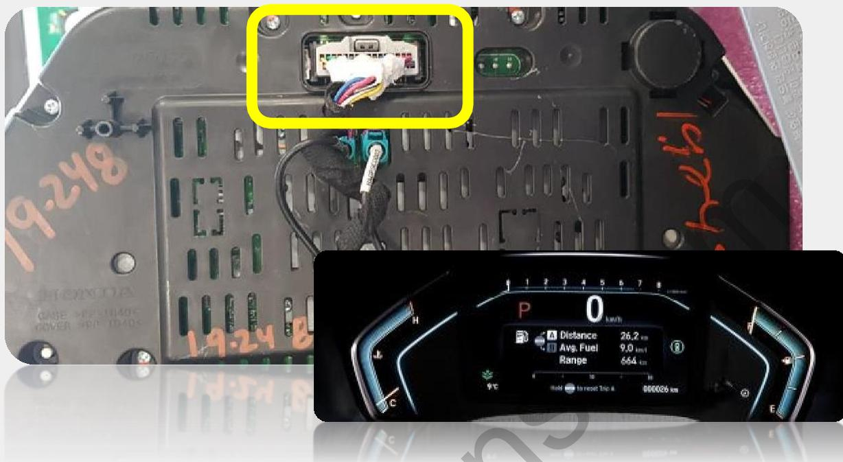
1. Please unplug above highlighted OEM Power/CAN cable from the Instrument monitor.
