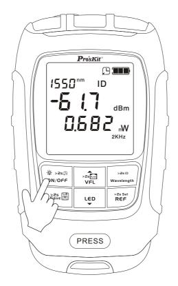
Optical power meter and Offset(self-calibration)Setting
