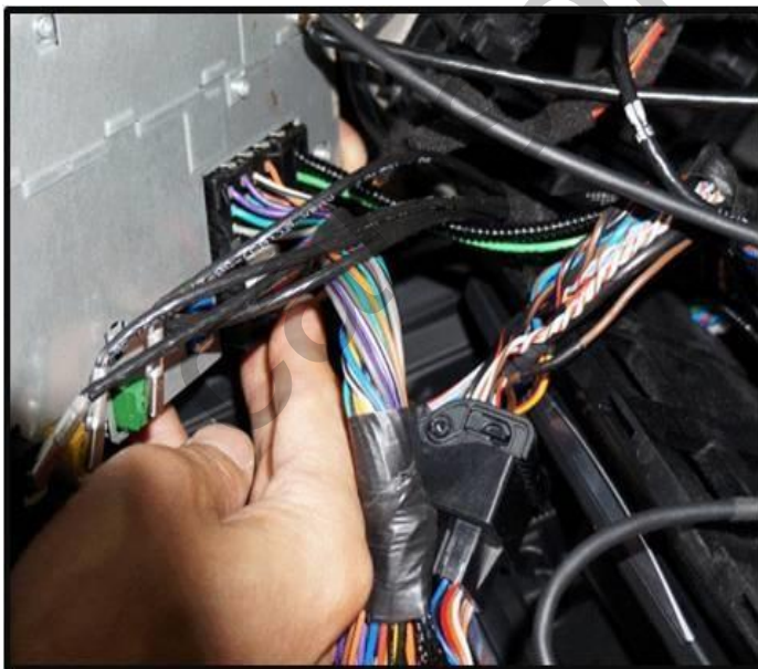
3. Connect the offered power cable to the back of command
