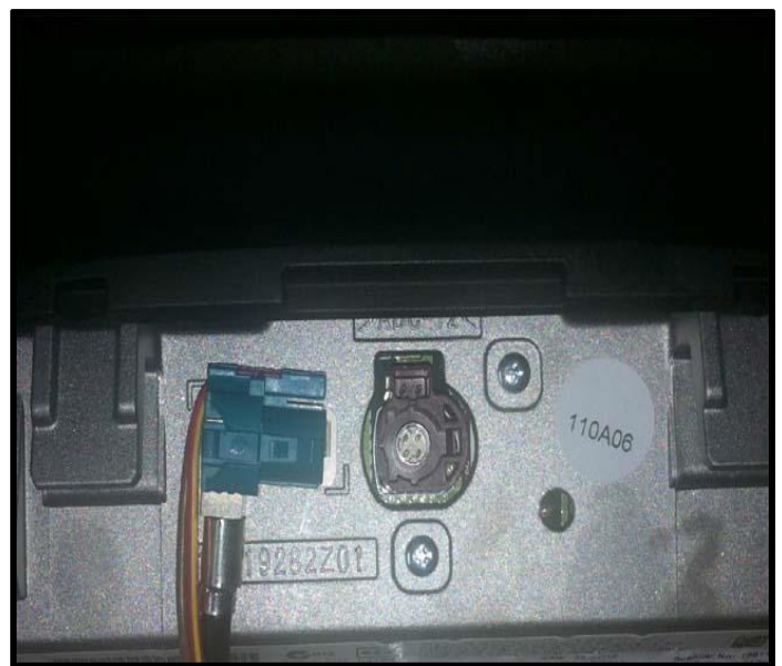
4. Connect the offered LVDS cable to the OEM monitor
