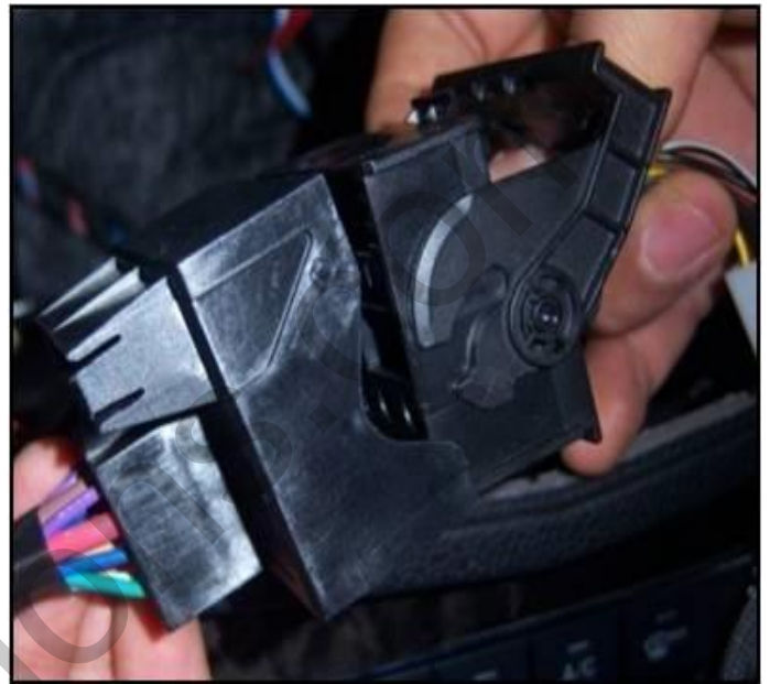
2. Connect the offered power cable to the OEM power cable
