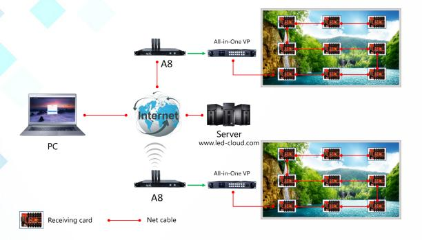
2. Asynchronous control: update programs through network cable connection, Wi-Fi connection and U disk. LAN Control support network cable connection and Wi-Fi bridge connection.
