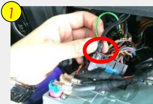
Pull out the bunch of cables from the backside of command and disconnect the marked optical fiber cable
