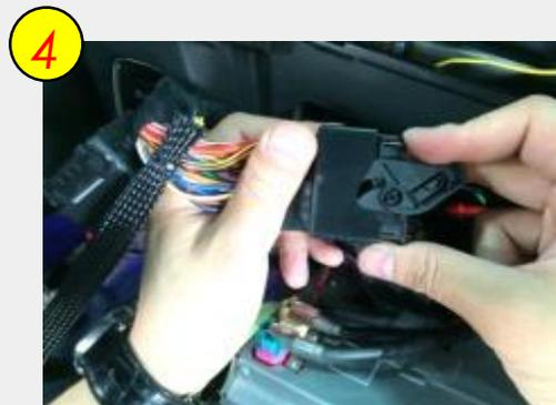
Connect the bunch of original cables to the provided power cable (Female connector)
