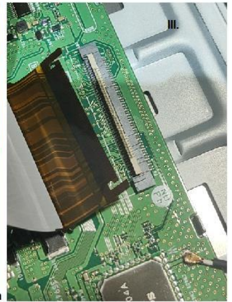
Then connect with the terminals on the screen panel,it's finished the flat cable connection as photo III .
