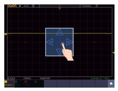
When the **M** and **V** icons appear, in the full screen, swipe left/right to change the time base, swipe up/down to change the voltage division of the selected channel. Click the icons to fine-turn, long-press to adjust continuously.
