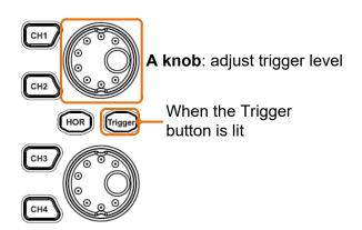
Figure 3-12 Trigger Control Zone
