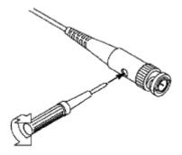
Figure 3-7 Adjust Probe
