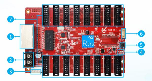
①: Gigabit Ethernet port, used to connect the sending card or receiving card, the same two network ports are interchangeable,
