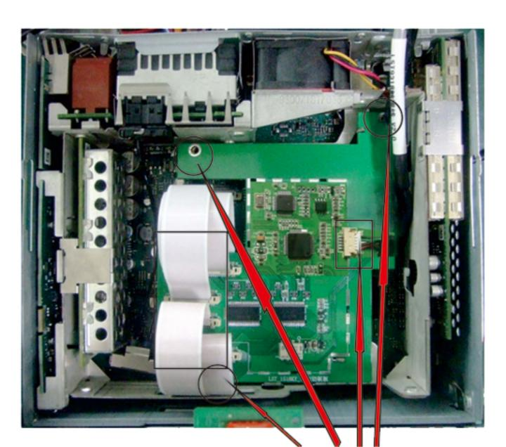
2,sub-board installation.connect well with 2PCS FPC and LVDS cable.
