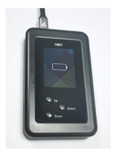
When you connect the battery, the programmer will automatically detect the chip used in the battery and enter the main menu.
