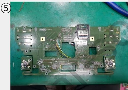
Please remove OEM resistances and do soldering some points with supplied cable on OEM PCB. Please refer to next page for the details.
