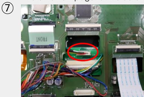
Please connect the cable to sub board. support@car-solutions.com soldered OEM PCB.
