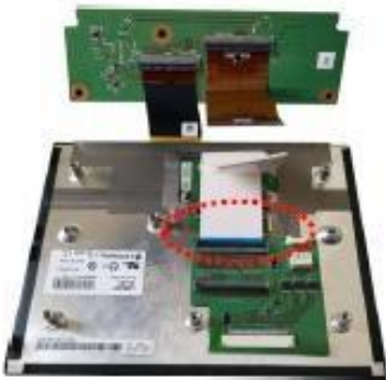
On the provided sub-board Connecting the Supplied FFC Cable (Connect so that the blue part is visible)
