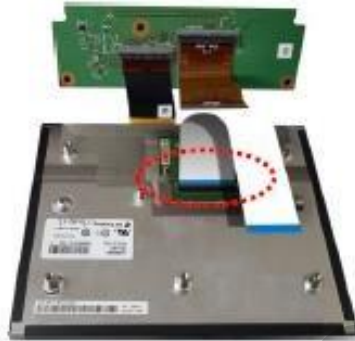
Where the original FPC cable is removed Connecting the Supplied FFC Cable (Connect so that the blue part is visible)
