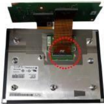
Original FPC cable removal
