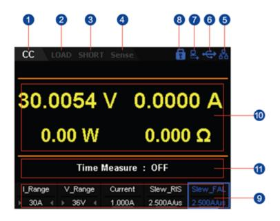
Figure 3: The user interface of the SDL1000X
