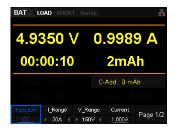
Figure 2-38 Battery Test Function Page 1
