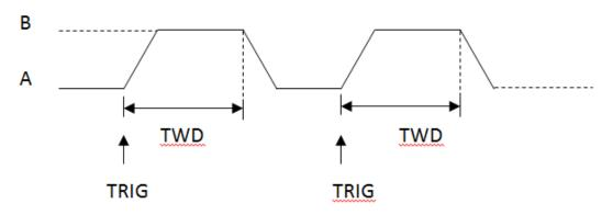
Figure 2-19 Transient CC Pulse Mode(Cont)
