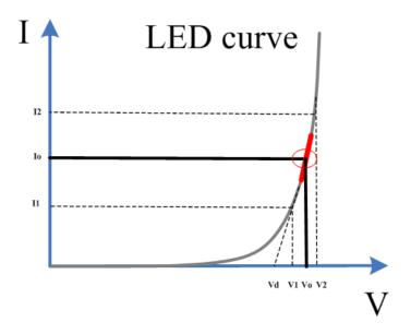
Figure 2-45 V - I characteristic curve of LEDs
