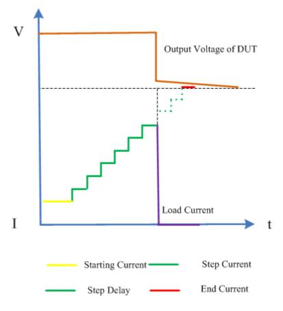
Figure 2-27 OCPT Test Function
