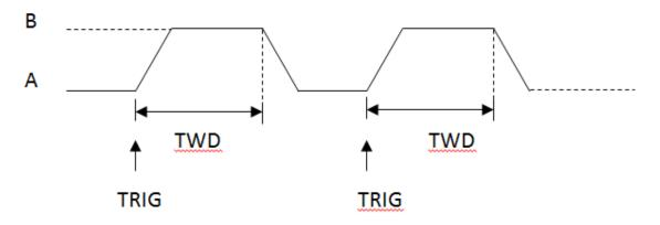
Figure 2-23 Transient CC Toggle Mode(Tog)
