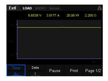
Figure 3-13 Waveform display interface of Extl mode
