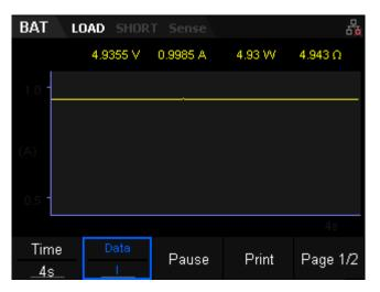
Figure 2-40 Waveform display interface of BAT
