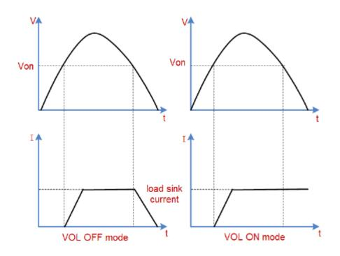
Figure 3-11 V - I characteristic curve of Von Latch
