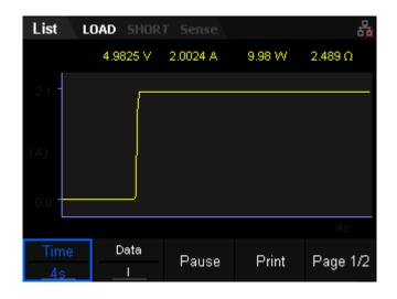
Figure 2-44 Waveform display interface of List mode
