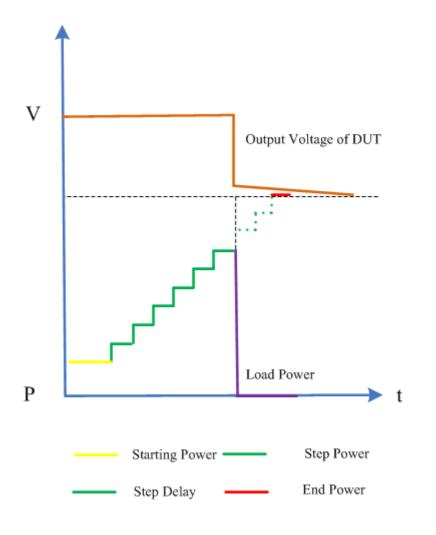
Figure 2-32 OPPT Test Function
