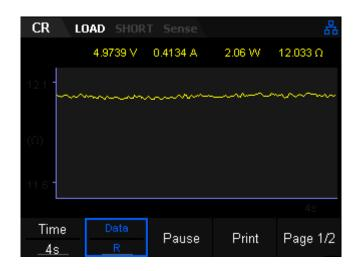
Figure 2-10 Waveform display interface of CR Mode
