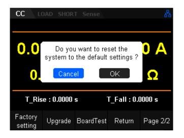
Figure 3-10 Restore factory setting interface
