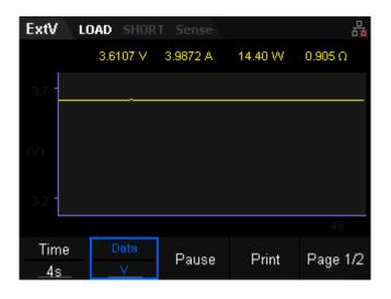
Figure 3-15 Waveform display interface of ExtV mode
