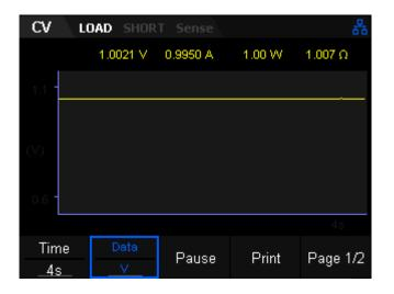
Figure 2-7 Waveform display interface of CV Mode
