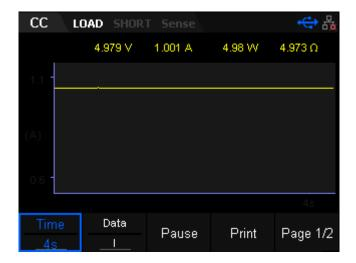
Figure 2-4 Waveform display interface of CC Mode
