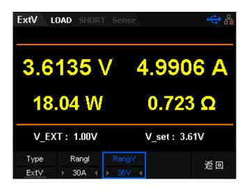
Figure 3-14 The main interface of the ExtV mode
