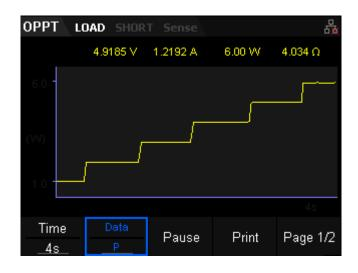
Figure 2-36 Waveform display interface of OPPT
