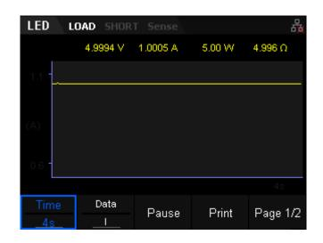
Figure 2-47 Waveform display interface of LED test mode
