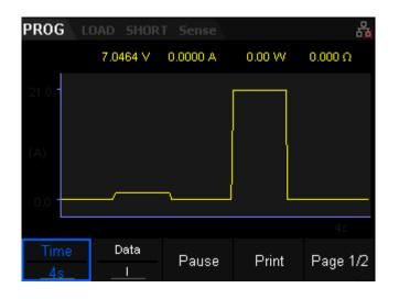
Figure 2-44 Waveform display interface of Program mode
