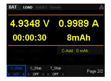
Figure 2-39 Battery Test Function Page 2
