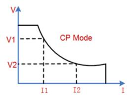
Constant power mode Figure 2-11 Voltage-Current Relationship Schema under CP Mode
