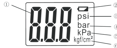
Figure 2 Display Symbols of LCD Screen
