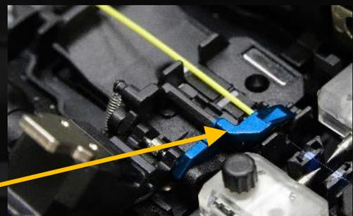
Time for opening wind protector and sheath clamp after splicing
