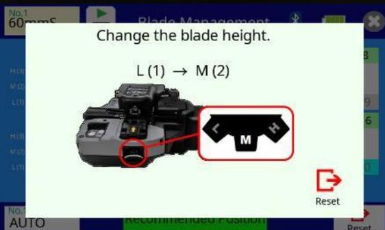
The screenshot shows the 86S fusion splicer interface with a table displaying blade management data:
