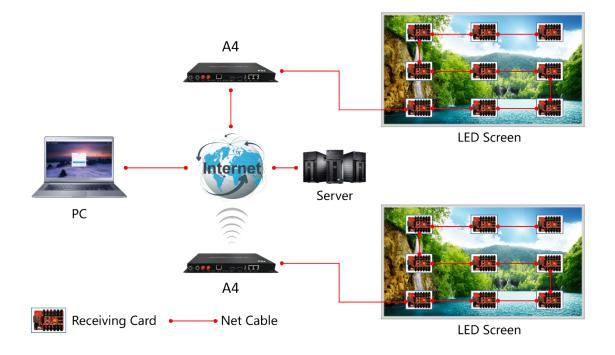
2. Asynchronous one-to-one control: Update programs by network cable connections, Wi-Fi connections or USB flash drives. LAN (cluster) control can access the LAN network through by network cable connection or Wi-Fi Bridge.
