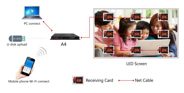
Real-time picture synchronization display: The play box is connected to the sync source through the HDMI high-definition video line, and the sync picture is automatically scaled without any setting.
