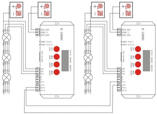
NOTE:1. When multiple controllers cascade, beginning from the second controller digital screen display 222, and status lights: on, off, on, off, strobe, all cascade controllers' playback speed controlled by
