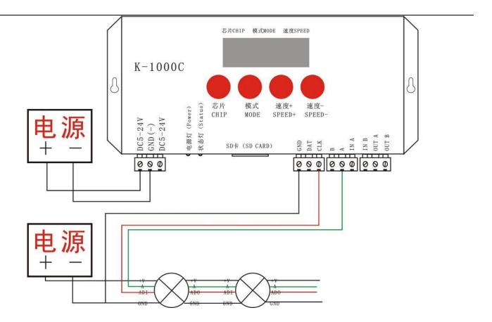
1. Like the above diagram, wired the line and start the controller, press "CHIP" and "MODE" at the same time switch to coding mode, adjust to Chip: 61 that is UCS512A or B coding mode, as below:
