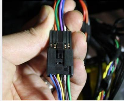
Connect the OEM connector to the supplied CAN IN/OUT
