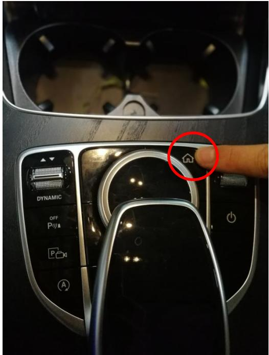
Please press main interface button for 2 seconds to exit 360, adjust to automatic parking.
