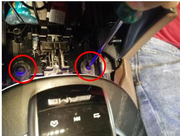
**3. Remove the handrail box and screws**
