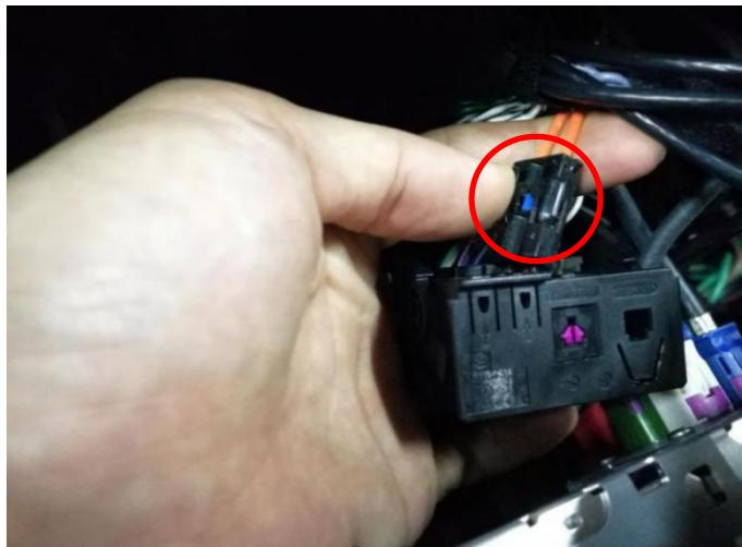
**6. Take off the transfer cables of head unit, plug fiber optic from OEM head unit and plug preserved position of camera interface box.**
