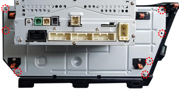
① Loosen all screws in the back of monitor
