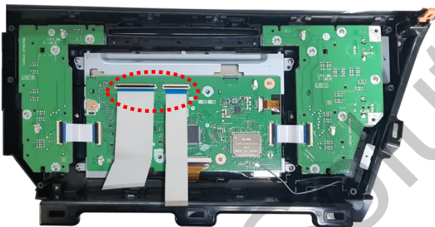
③ Connect the offered FFC cable to the OEM PCB board
