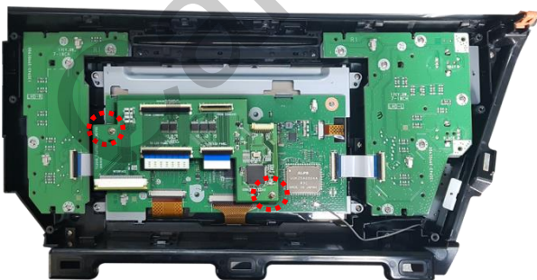
⑤ Using the offered washer bolt the indicated part
