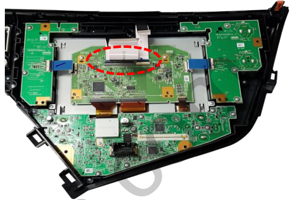
② Disconnect an OEM FPC cable from an OEM PCB board
