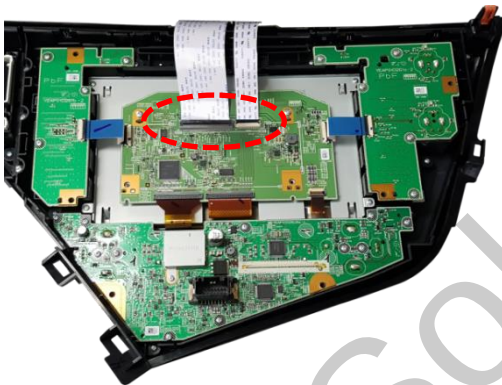
③ Connect the offered FFC cable to the OEM PCB board
