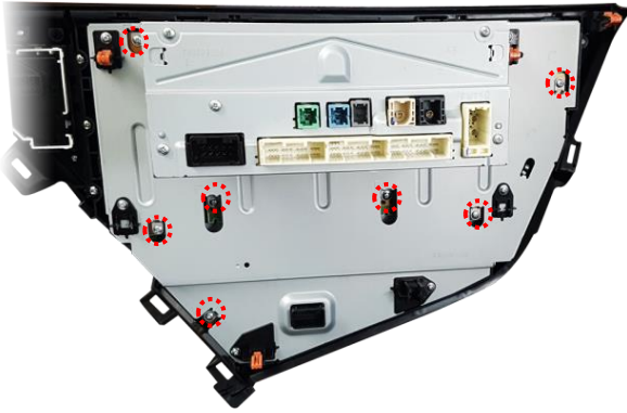
① Loosen all screws in the back of monitor
