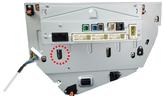
⑥ Before assembling the monitor, Put the LVDS cable into the hole as marked
