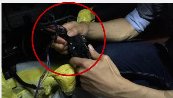
Connect a bunch of cables from the command to a female connector of Jack by jack cable.
