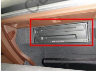
Use trim removal tools to take out of radio NTG5 main unit. (Position may be different based on car models.)
