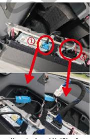
pull out plug (1) (2) of screen conrrespondingly connect to our plug take out screen and main unit then put our plug back to screen
