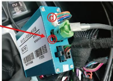
5. Finish interface harnesses on interface box;
