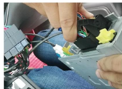
3. Connect the other end of interface Quad_Lock connector to original position on main unit.
