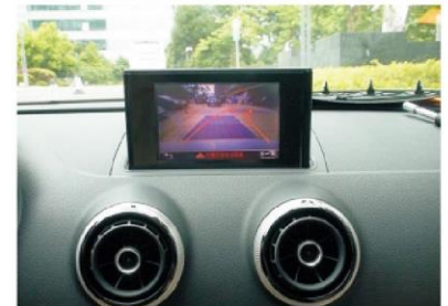
6. Performance of interface. (Auto-Display when shift into Reverse gear)
