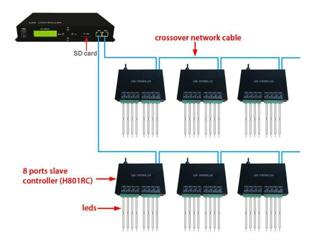
If you want to control for example WS2812B strip, just connect GND, DI on strip to GND, DAT on slave controller.
