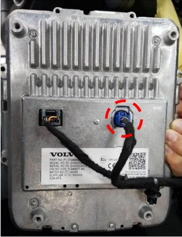
Find OEM blue cable on the back side of the monitor
