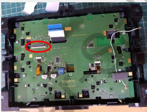
Remove the FFC cable from the marked place
