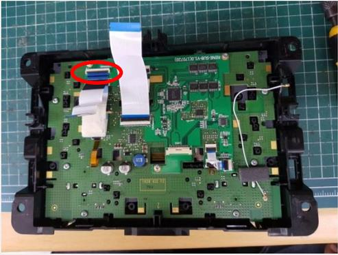
Connect the OEM FFC cable which was removed from 5 to marked place
