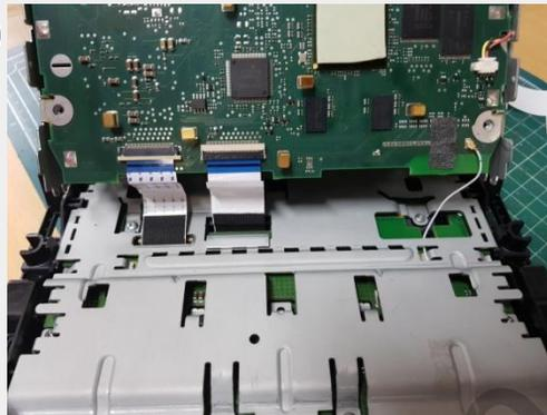
Disassemble the monitor and headunit
