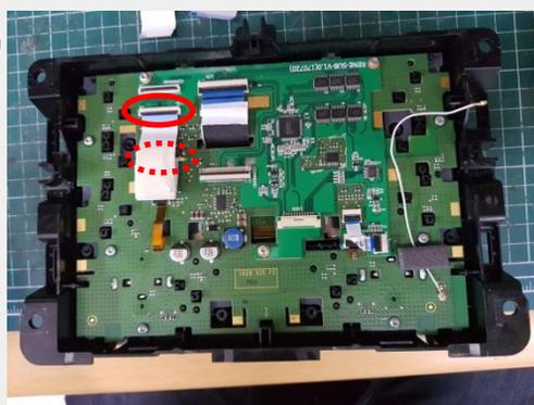
The supplied FFC cable shall be connected between OEM board and subboard
