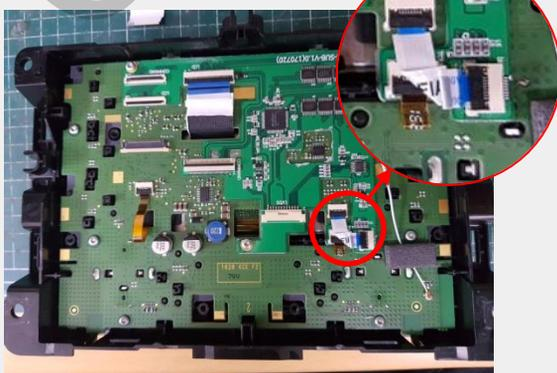
Connect the supplied touch FFC cable (90° curved shape)
