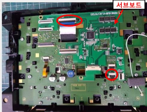
Place the supplied subboard on the marked place and connect OEM cables
