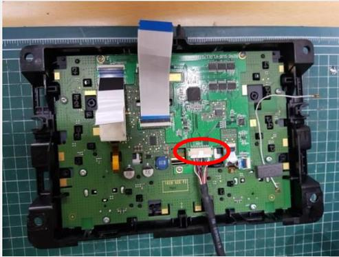
Connect LVDS cable to the marked place
