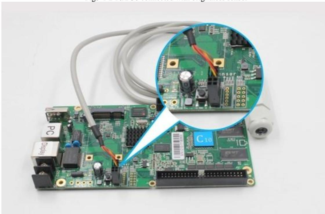
Fig3-2 C10/C30 connected with brightness sensor
