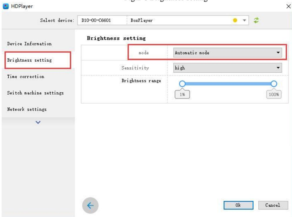
Fig.2-7 Brightness automatic mode
