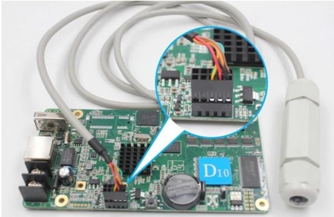
Fig3-1 D10/D30 connected with brightness sensor
