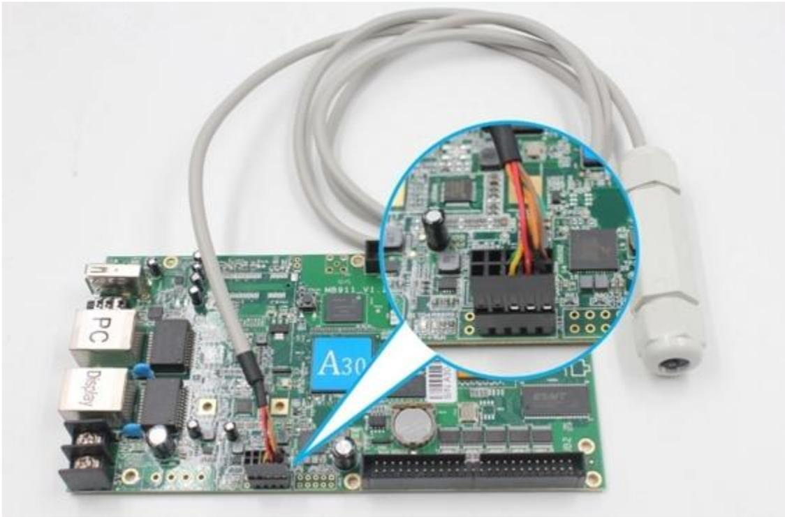
Fig3-3A30/A30+ connected with brightness sensor
