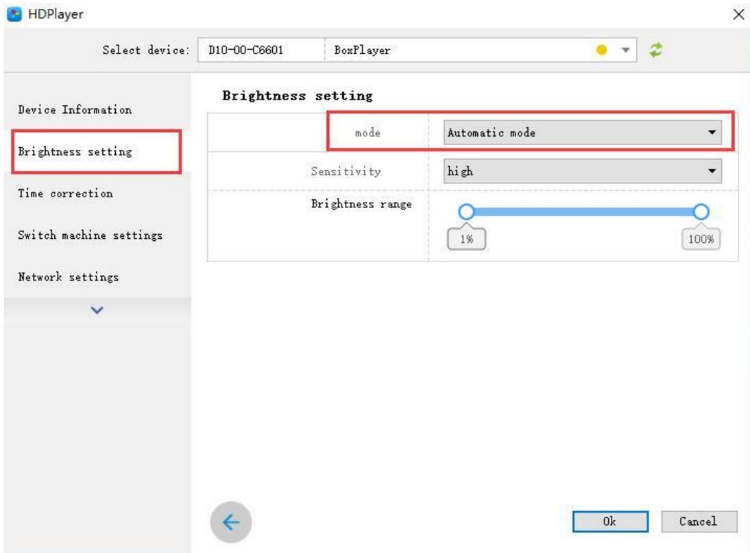
Fig3-4 Brightness automatic mode
