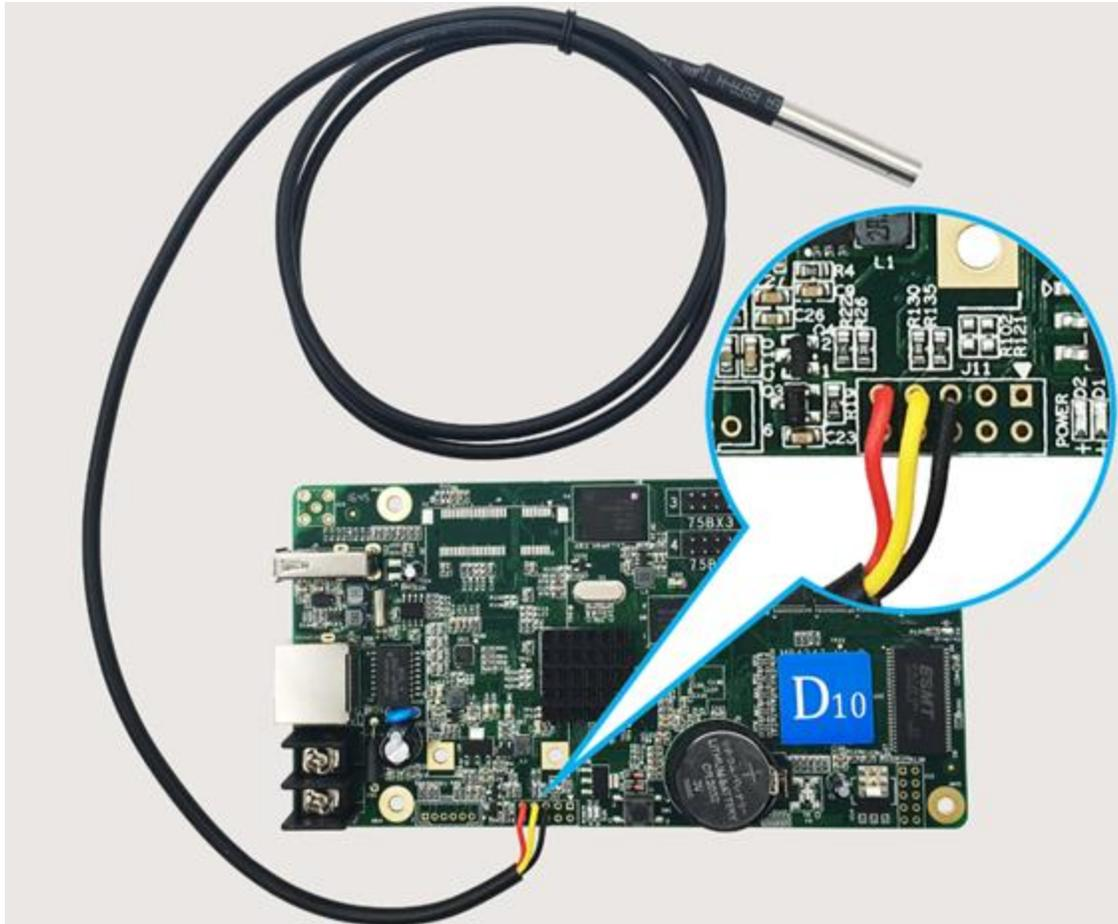
Fig.1-1 D10/D30connected with temperature sensor
