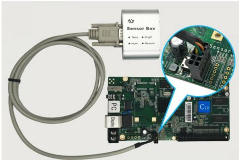
Fig.2-1 the connection of C10/C30 and sensor box
