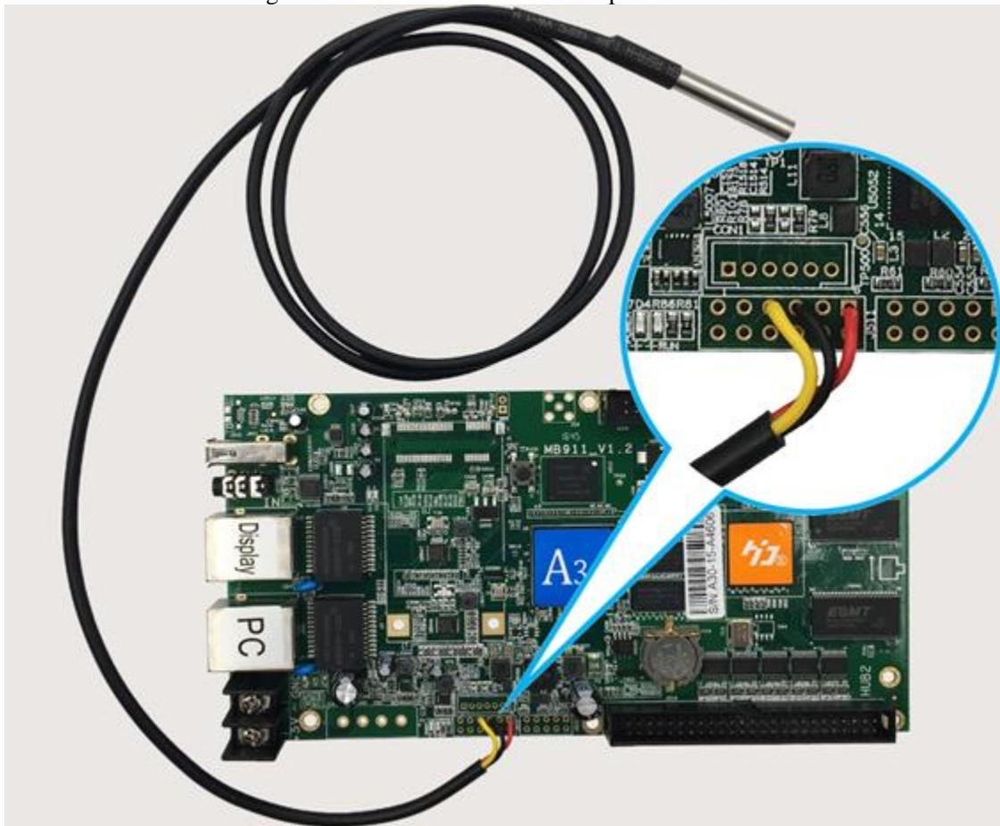
Fig1-3 A30connected with temperature sensor
