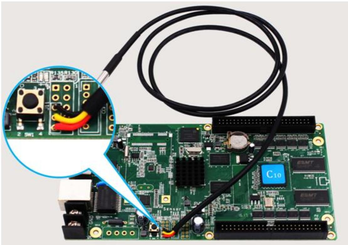
Fig.1-2 C10/C30connected with temperature sensor
