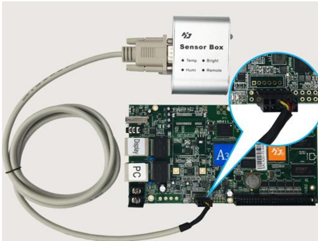
Fig.2-3 the connection of A30/A30+ and sensor box
