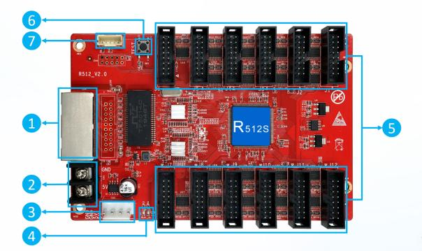
(1): Gigabit Ethernet port, used to connect the sending card or receiving card, the same two network ports are interchangeable,
