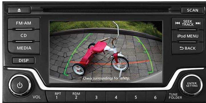
Depending on the camera view angle and the place of installation, parking lines may not be informative and will then need to be adjusted in the diagnostic menu of the car radio.
