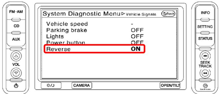
Press the **BACK** button in the top right corner to exit the diagnostics menu.
