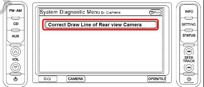
Image from the connected camera will be activated with OSD buttons for adjustment of parking lines and camera image. Align parking lines relative to the center of the image and adjust the lines accordingly.
