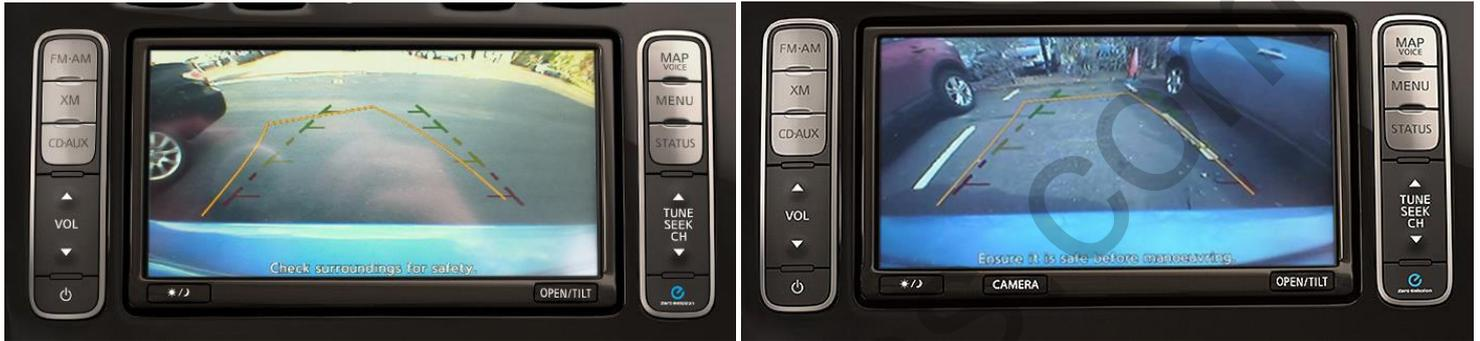
Depending on the camera view angle and the place of installation, parking lines may not be informative and will then need to be adjusted in the diagnostic menu of the car radio.
