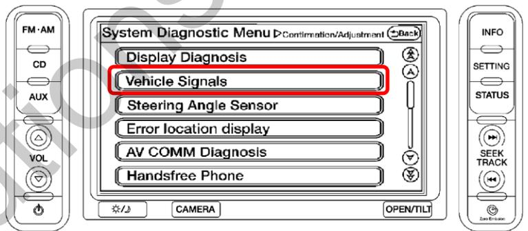
Check the **Reverse** signal in the dialog window that appears. **ON** message should appear on the screen when you switch to reverse, and disappear when you switch back. If this does not happen (there's no message or it does not react), use the grey **REV wire** of our cable.
