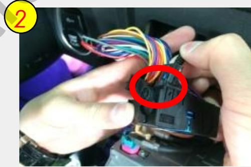
Connect the optical fiber cable to the supplied power cable
