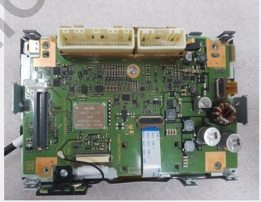
Place the board on the top of the metal case and reassemble the rest parts
