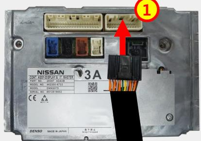
※ Remove OEM cable from ① connector of monitor behind and connect OEM cable to supplied power cable the other side of supplied connector shall be connected to ① connector
