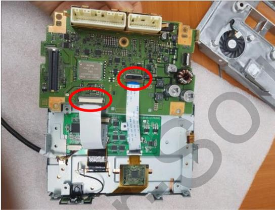
The opposite side of supplied FFC cables should be connected to the place where OEM FPC cables are connected
