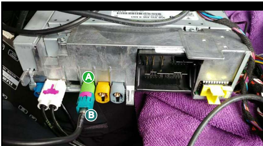
1. PLEASE PULL OUT OEM LVDS CABLE (A), AND LVDS IN CABLE (B) OF INTERFACE CONNECT WITH OEM (A).
