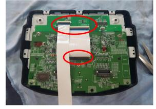
Connect the supplied FFC cables like picture above
