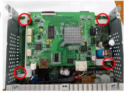
Place the supplied interface on the top of the OEM board and screw bolts again
