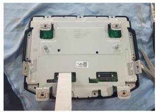
Pull out a long FFC cable through a hole and reassemble the metal cover
