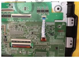
The touch cable shall be connected between the supplied subboard and the OEM board where original touch cable is connected
