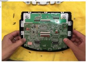
Reassemble the OEM board on the top of the subboard
