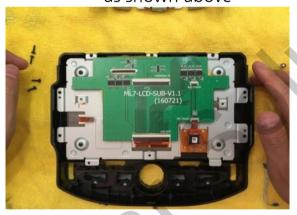
Place the subboard on the top and connect FPC cable
